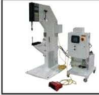
Universal presses are hydraulically operated presses that easily adapt to join a variety of parts.
