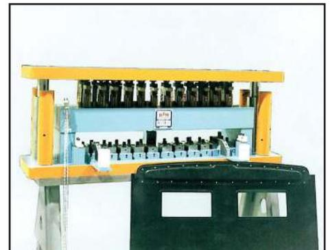
Tog-L-Loc® "bump" die for joining prepainted aluminum sunroof.
